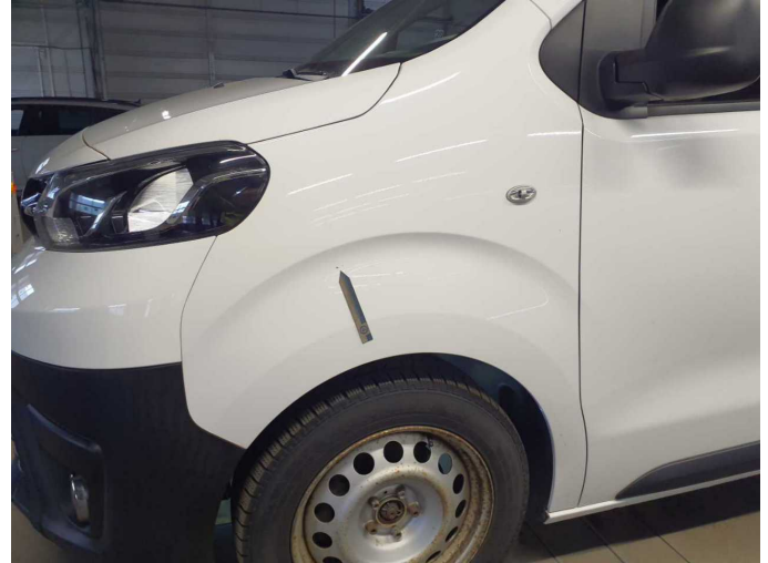
Damage 2: Mudguard - left side: Mudguard - left side - Stone chips - Smart repair
