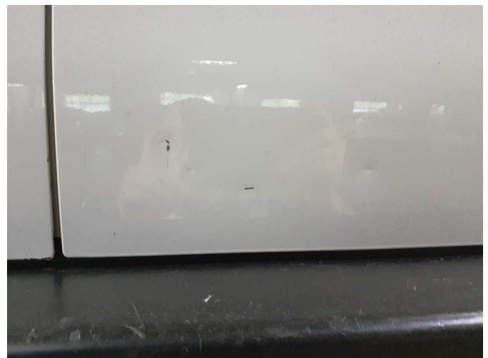
Damage 7: Boot lid / rear door: Rear door - right side - Dent / paintcoat damage - Repair and paint
