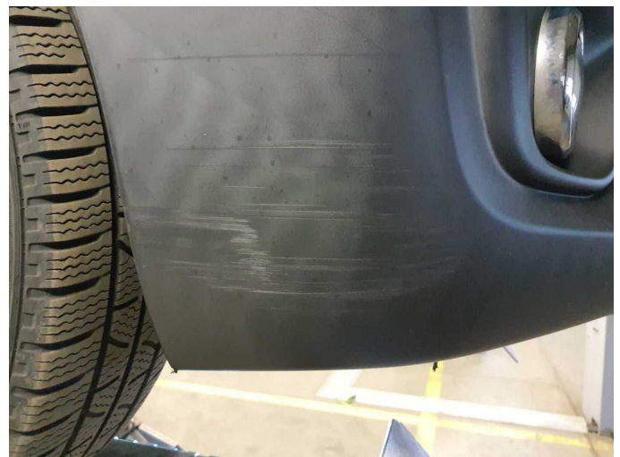
Damage 6: Front bumper: Front bumper (Zierleisten) - Scratched - Smart repair
