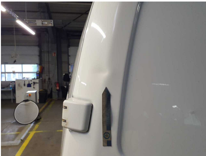
Damage 4: Boot lid / rear door: Rear door - left side - Deformed - Smart repair
