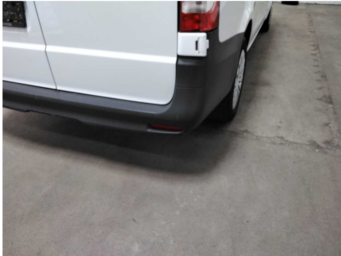
Damage 5: Rear bumper: Rear bumper - Scratch(es) - Replace
