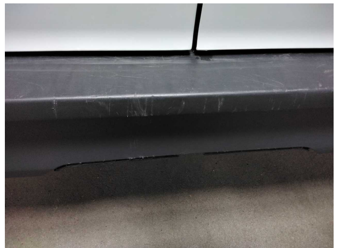
Damage 5: Rear bumper: Rear bumper - Scratch(es) - Replace
