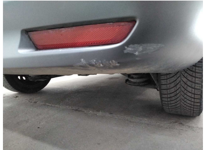
Damage 5: Rear bumper: Rear bumper - Scratch(es) - Replace
