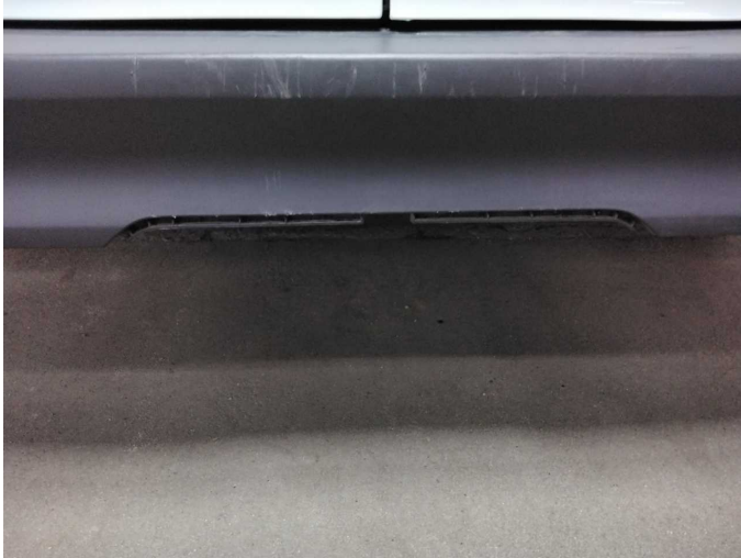
Damage 2: Rear bumper: Rear bumper (Blende) - Missing - Replace
