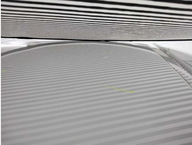
Damage 4: Roof: Roof - dent(s) - Smooth repair work
