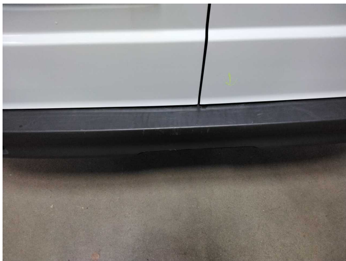
Damage 5: Rear bumper: Rear bumper - Scratch(es) - Replace
