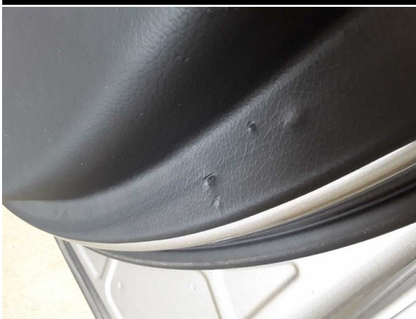
Damage #7: Trim / covers: Door trim - front right side - Damaged - Replace
