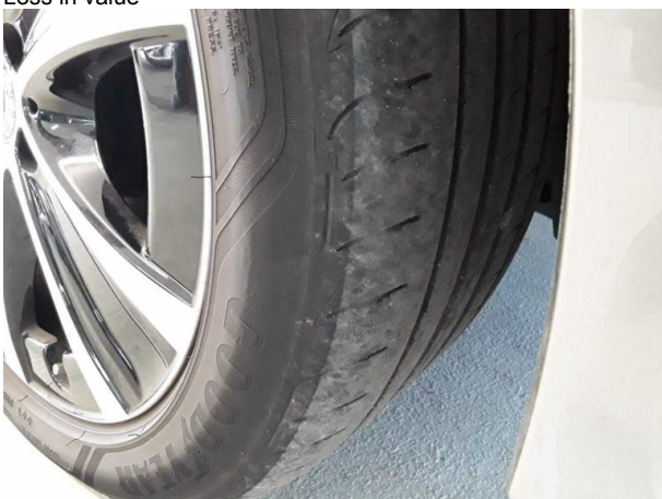
Damage #6: Wheel / tyres: Tyre - front - Worn - Replace
