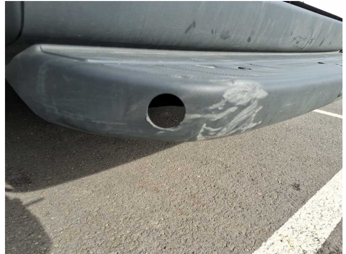
Damage 2: Rear bumper: Parking sensors - left side (Außen, inkl. Halter) - Missing - Replace
