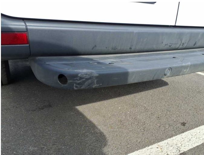
Damage 2: Rear bumper: Parking sensors - left side (Außen, inkl. Halter) - Missing - Replace
