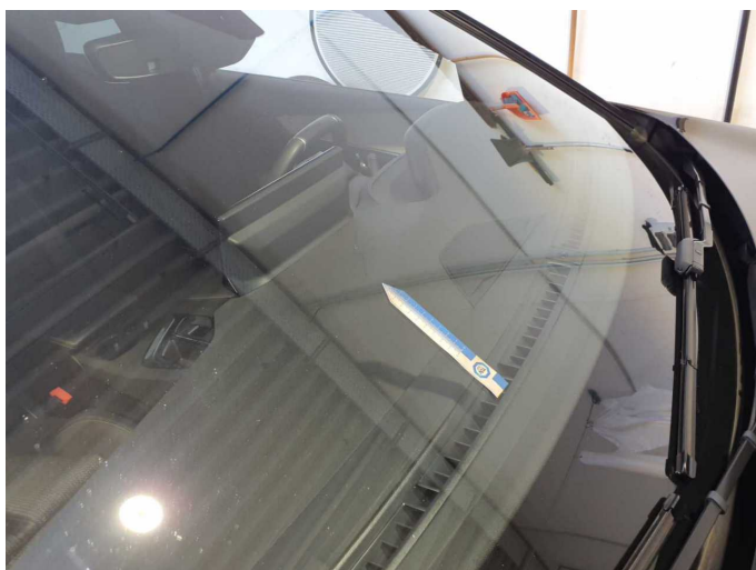
Damage 9: Vehicle glazing: Windscreen - Broken / torn - Replace
