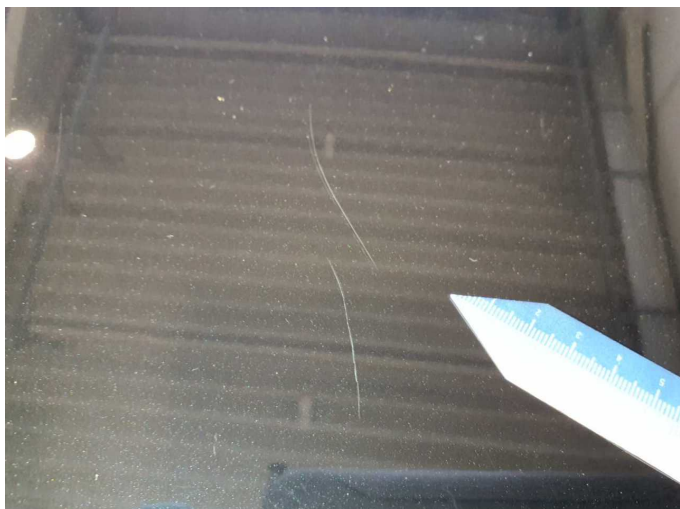
Damage 7: Bonnet: Bonnet - Scratch(es) - Paint
