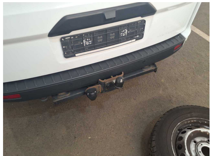
Damage 1: Rear of vehicle: Trailer hitch - Corrosion - Loss in value
