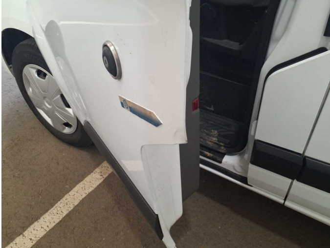
Damage 3: Door - front left side: Door - Deformed - Repair and paint
