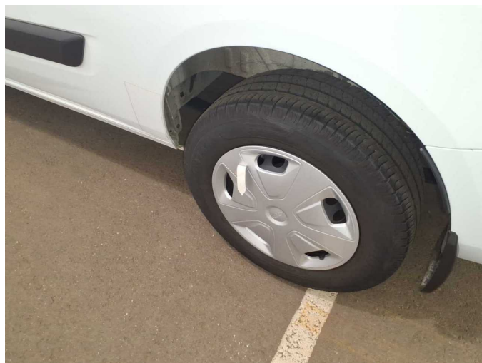
Damage 2: Wheel / tyres: Tyre - rear left side (nicht fahrbereit) - Broken / torn - Replace
