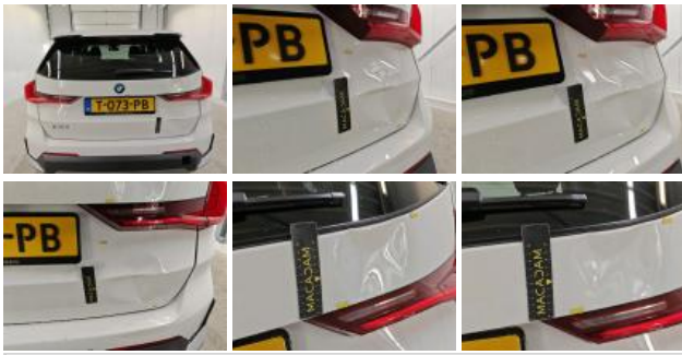
Rear light R tailgate, Crack, Replace
