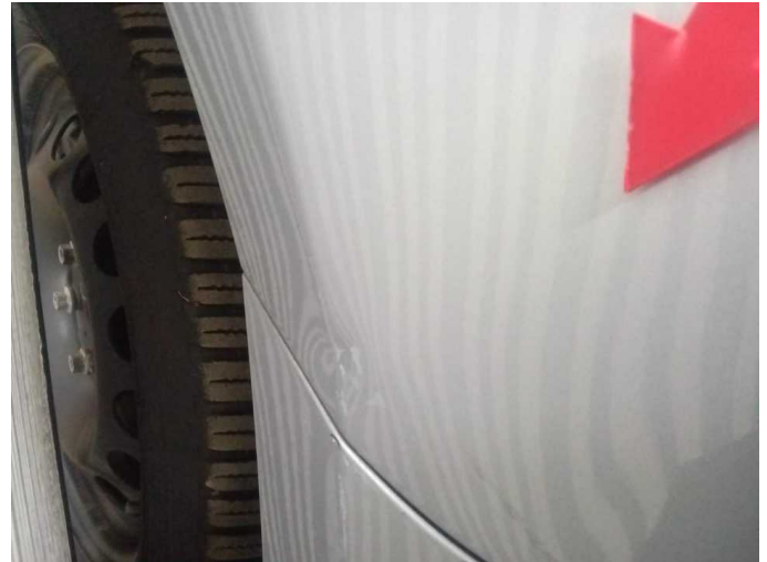
Damage 7: Mudguard - right side: Mudguard - right side - Dent / paintcoat damage - Replace
