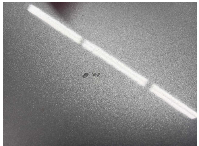
Damage 6: Bonnet: Bonnet - Stone chips - Paint
