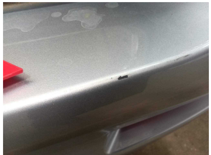
Damage 4: Rear bumper: Rear bumper - Scratch(es) - Paint
