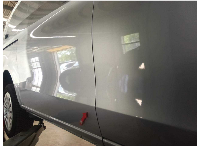
Wear and tear 9: Sliding door, right: Sliding door - dent(s) - No deduction
