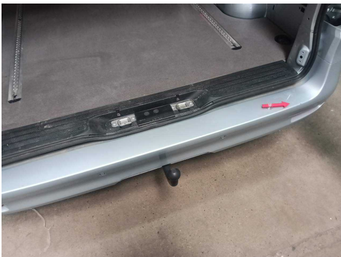
Damage 4: Rear bumper: Rear bumper - Scratch(es) - Paint
