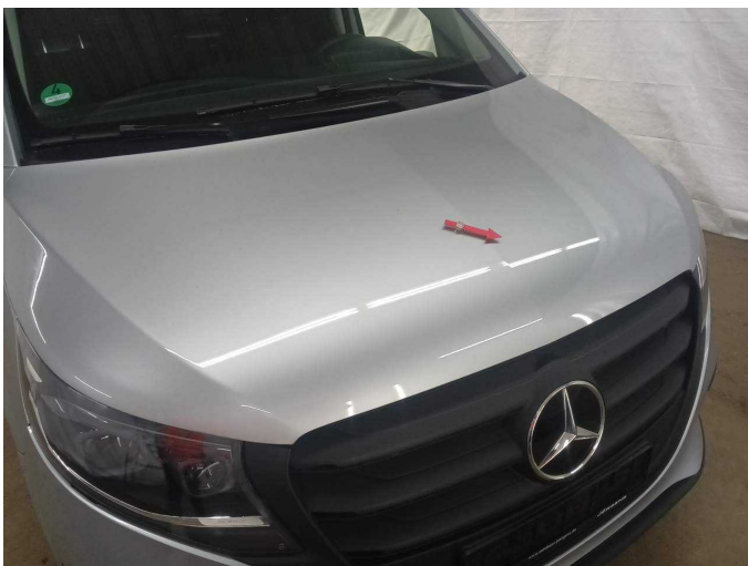
Damage 6: Bonnet: Bonnet - Stone chips - Paint
