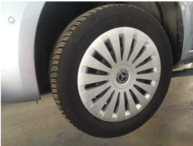
Damage 3: Wheel / tyres: Tyre - front (Allwetterreifen) - Porous / cracked - Replace
