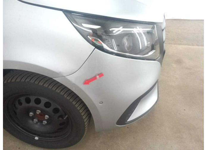
Damage 5: Front bumper: Front bumper - Scratch(es) - Paint
