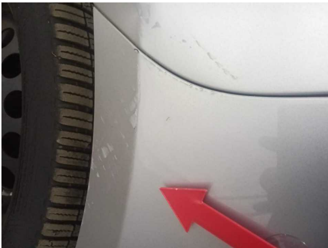
Damage 5: Front bumper: Front bumper - Scratch(es) - Paint
