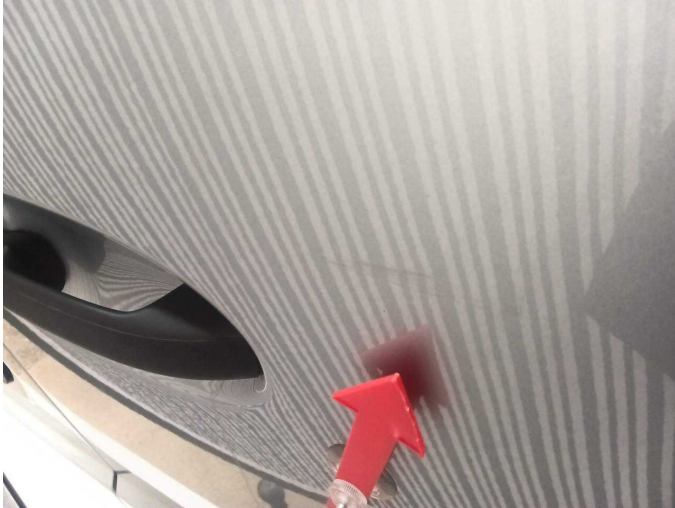
Damage 8: Boot lid / rear door: Boot lid - Dent / paintcoat damage - Repair and paint
