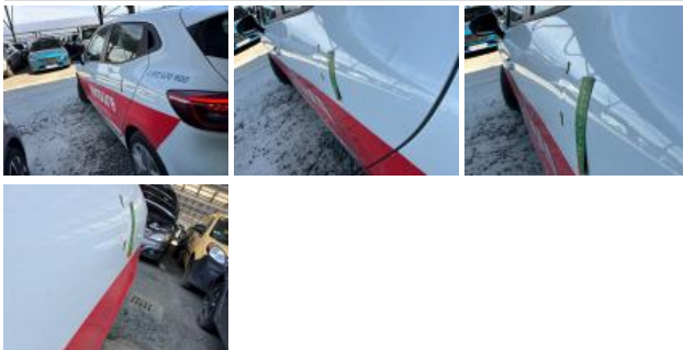
Wing RL, Dent(s), Repair and paint (complete)
