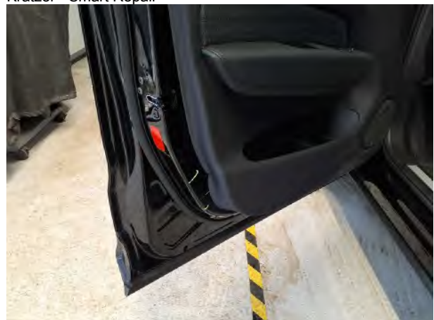
Beschädigung #11: Tür vorn links: Tür (innen) - Delle / Lackschaden - Smart Repair
