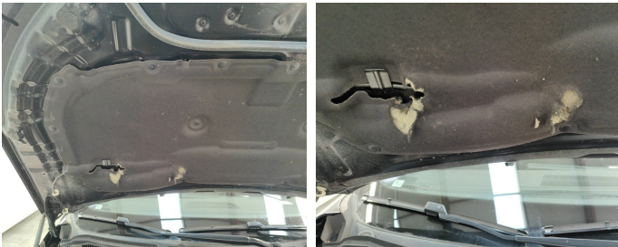
Front Bonnet / Insulation / Replace-cracked
