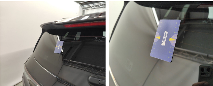
Rear Bonnet / Rear Window / Replace-scratch
