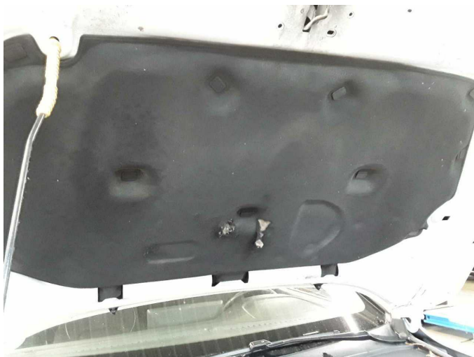
Damage 2: Bonnet: Insulation lining - Damaged - Replace
