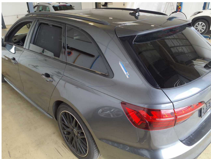
Damage 4: Body: D-pillar - left side - dent(s) - Smart repair
