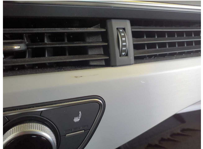
Damage 6: Instrument panel: Instrument panel (Blende Schalttafel) - Scratch(es) - Replace
