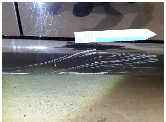
Damage 3: Sill - right side: Trim - Scratch(es) - Paint
