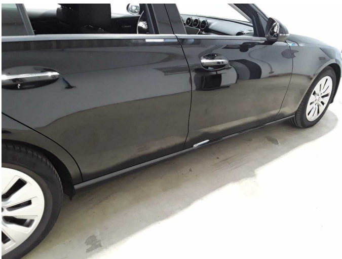
Damage 3: Sill - right side: Trim - Scratch(es) - Paint
