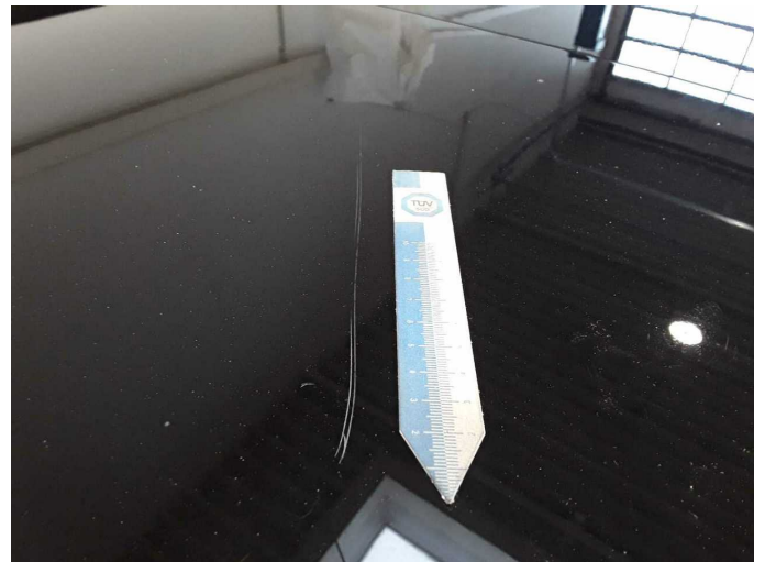
Damage 8: Roof: Roof - Scratch(es) - Paint
