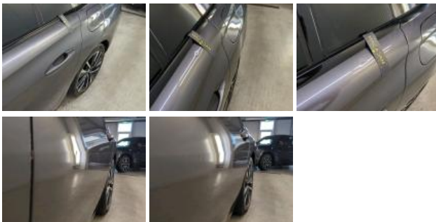
Wing RL, Rust, Repair and paint (complete)
