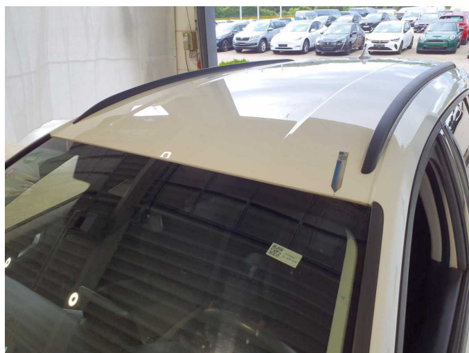
Damage 4: Roof: Roof (Dachkante) - Corrosion - Paint
