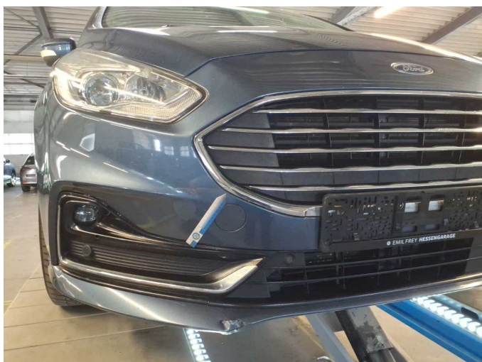
Damage 18: Bonnet: Radiator grille - Damaged - Replace
