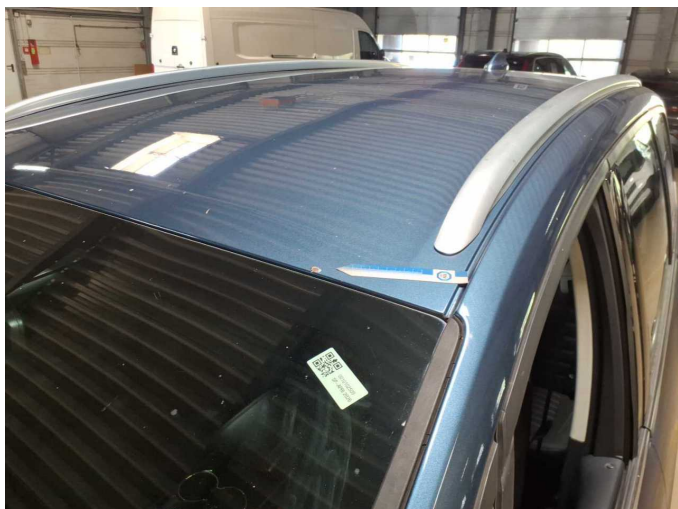
Damage 17: Roof: Roof - Corrosion - Smart repair
