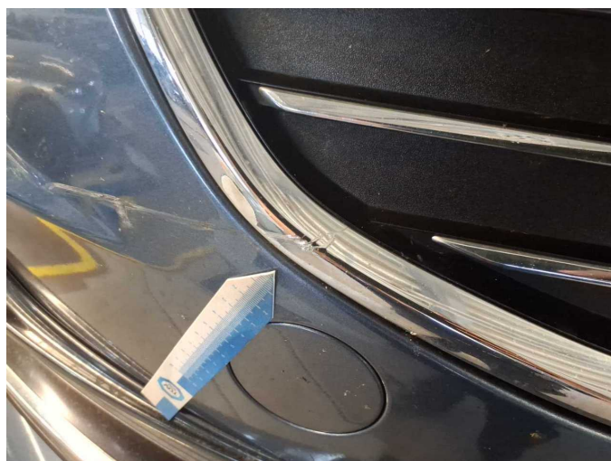
Damage 18: Bonnet: Radiator grille - Damaged - Replace
