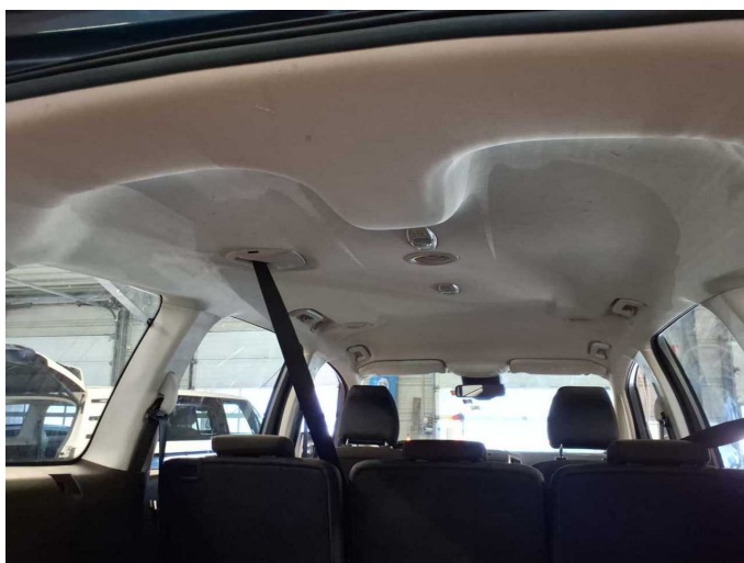
Damage 19: Trim / covers: Roof lining - Scratched - Loss in value
