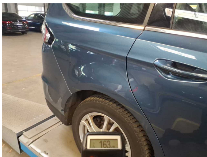
Repainting 2: Side panel - rear right side
