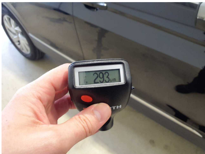
Repainting 3: Door - front right side
