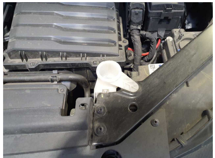
Damage 1: Screen cleaning: Cover washing container - Missing - Replace
