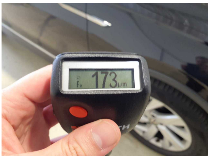
Repainting 2: Mudguard - right side
