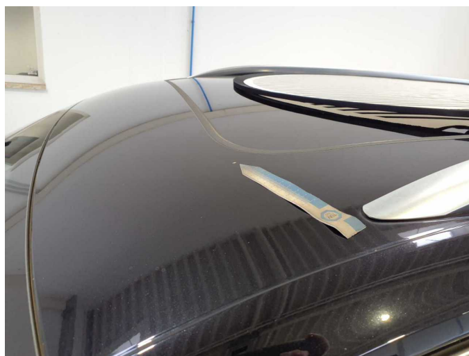
Damage 12: Roof: Roof - Corrosion - Paint
