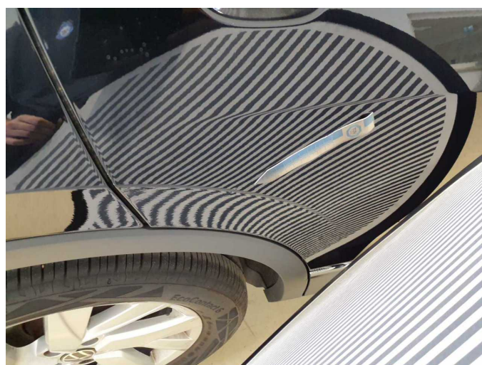
Damage 5: Door - rear right side: Door - dent(s) - Smart repair
