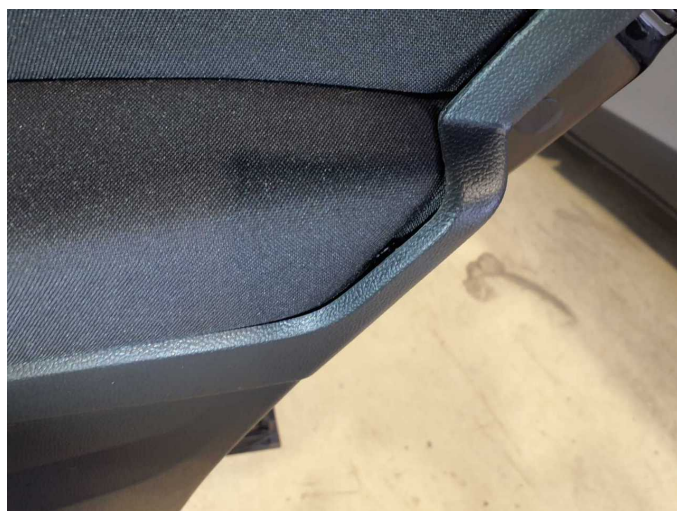
Damage 10: Trim / covers: Door trim - rear right side - Broken / torn - Replace
