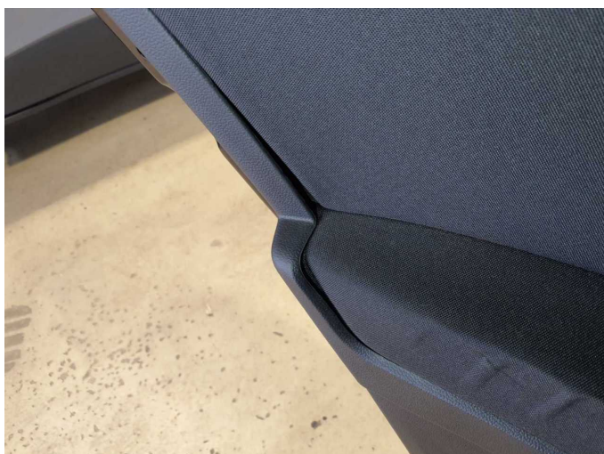
Damage 9: Trim / covers: Door trim - rear left side - Broken / torn - Replace
