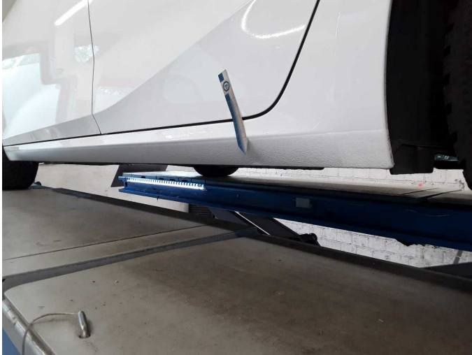
Wear and tear 4: Sill - left side: Sill - dent(s) - No deduction
