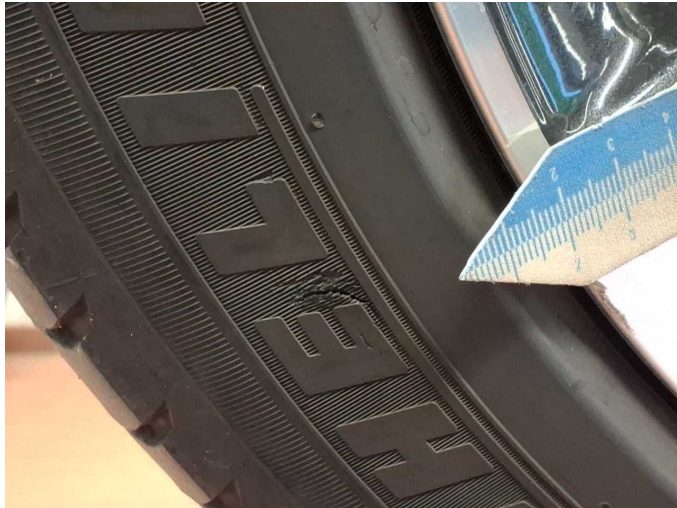
Damage 4: Wheel / tyres: Tyre - front left side - Broken / torn - Replace
