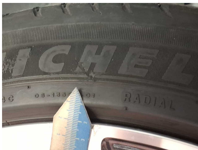
Damage 3: Wheel / tyres: Tyre - rear right side - Broken / torn - Replace
