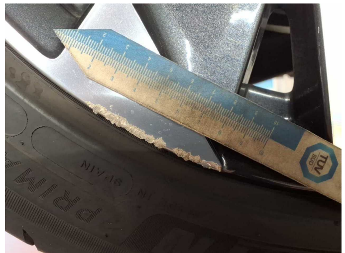
Damage 7: Wheel / tyres: Alloy rim - rear right side - Scratched - Replace
