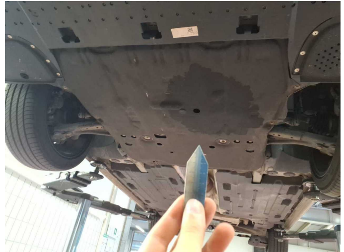
Damage 5: Engine: Engine - Leaking - Perform diagnosis
