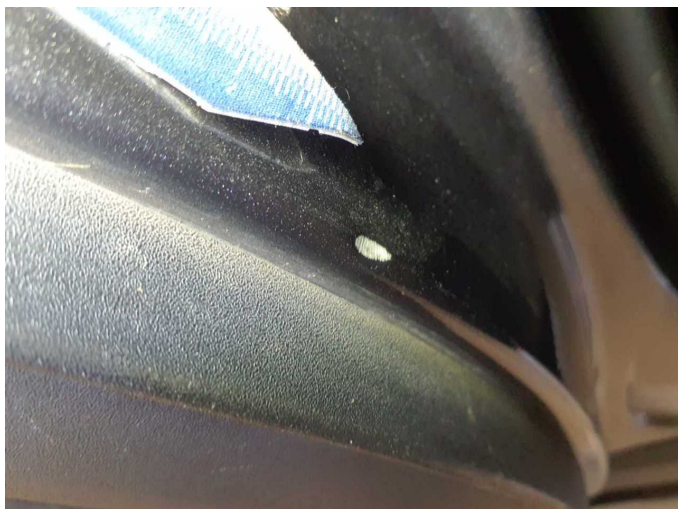
Damage 5: Side panel - rear right side: Sill - Scratch(es) - Smart repair
