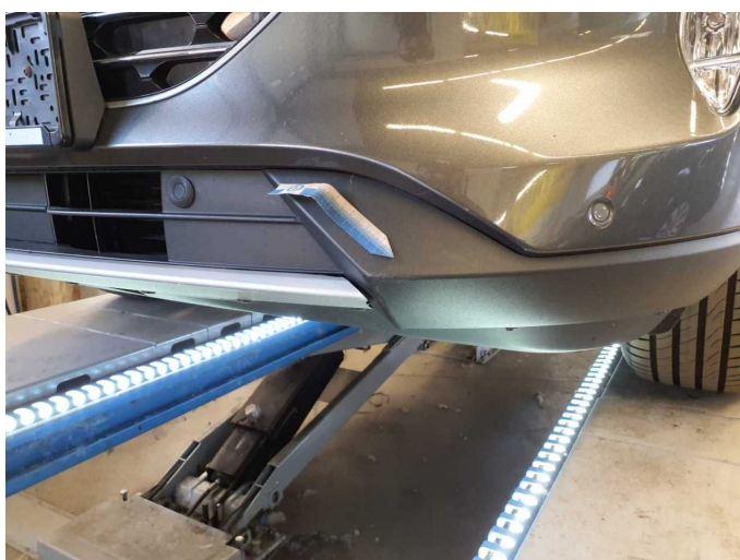
Damage 6: Front bumper: Spoiler (+Blende) - Damaged - Replace
