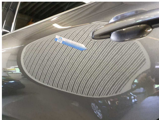
Damage 7: Door - rear left side: Door - Unprofessionally repaired - Repair and paint
