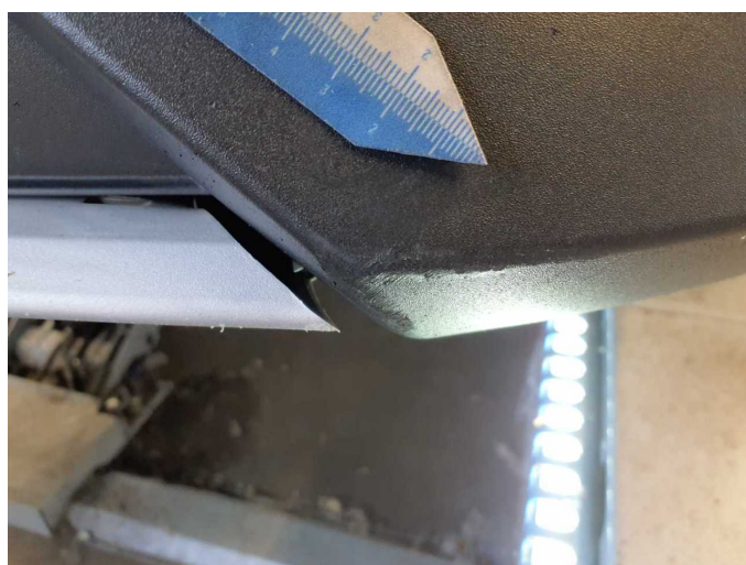
Damage 6: Front bumper: Spoiler (+Blende) - Damaged - Replace
