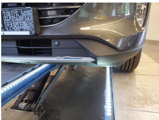
Damage 6: Front bumper: Spoiler (+Blende) - Damaged - Replace
