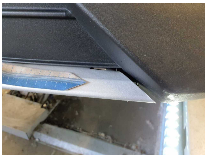
Damage 6: Front bumper: Spoiler (+Blende) - Damaged - Replace
