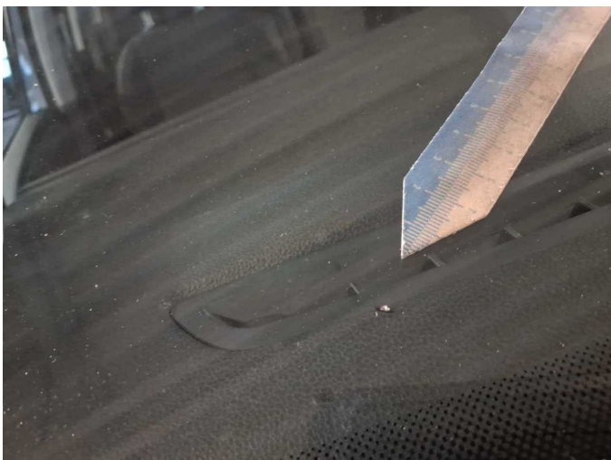
Damage 7: Vehicle glazing: Windscreen - Stone chips - Replace
