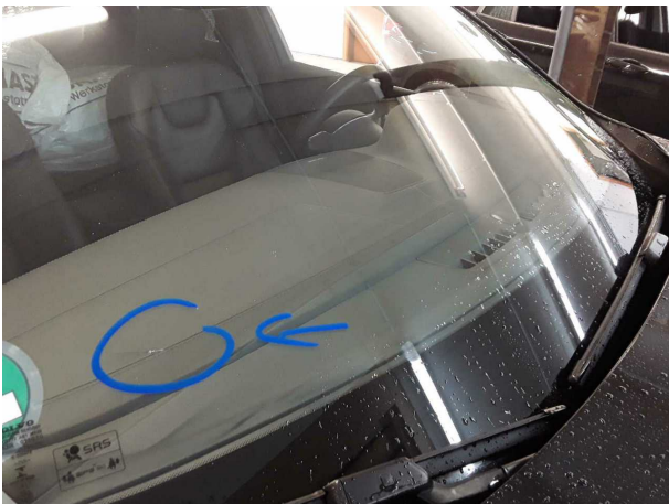
Damage #3: Vehicle glazing: Windscreen (Rissbildung) - Replace
