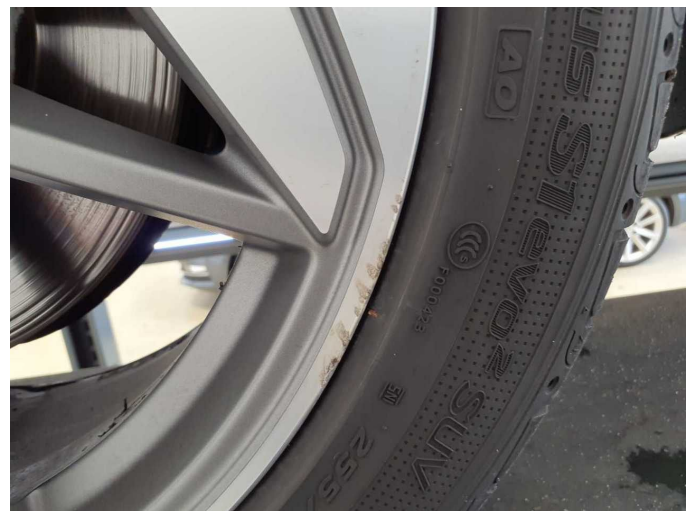
Damage 11: Wheel / tyres: Alloy rim - front left side - Corrosion - Replace
