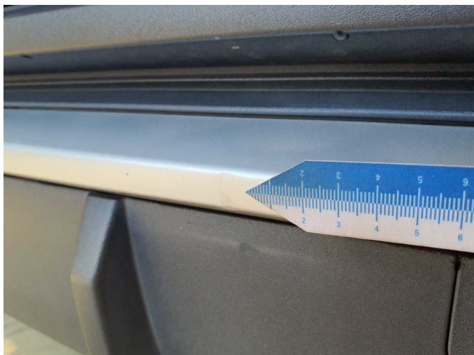
Damage 2: Rear bumper: Rear bumper (unpainted) (Blende) - dent(s) - Replace
