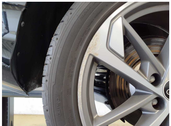
Damage 10: Wheel / tyres: Alloy rim - rear right side - Corrosion - Replace
