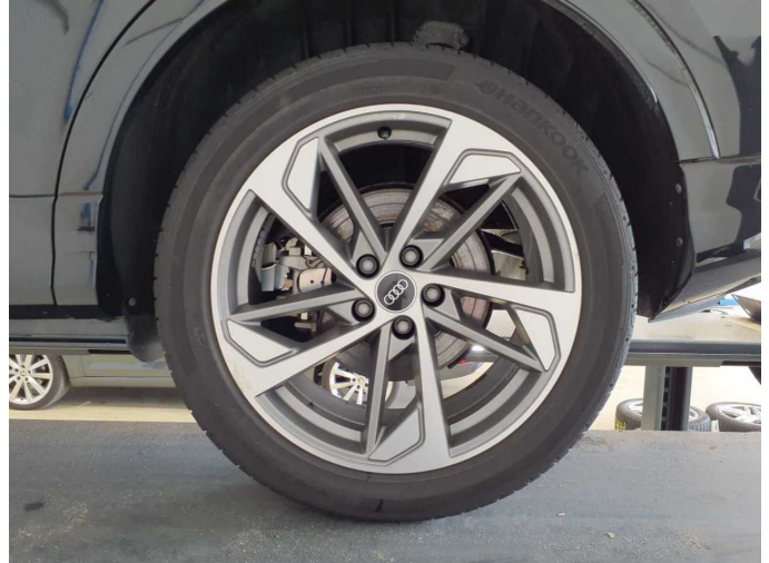
Damage 9: Wheel / tyres: Alloy rim - rear left side - Corrosion - Replace
