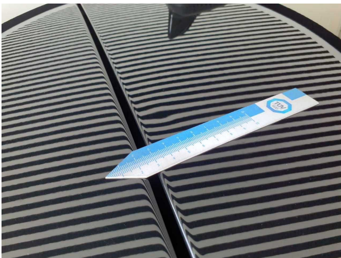
Damage 1: Roof: Roof - dent(s) - Smooth repair work
