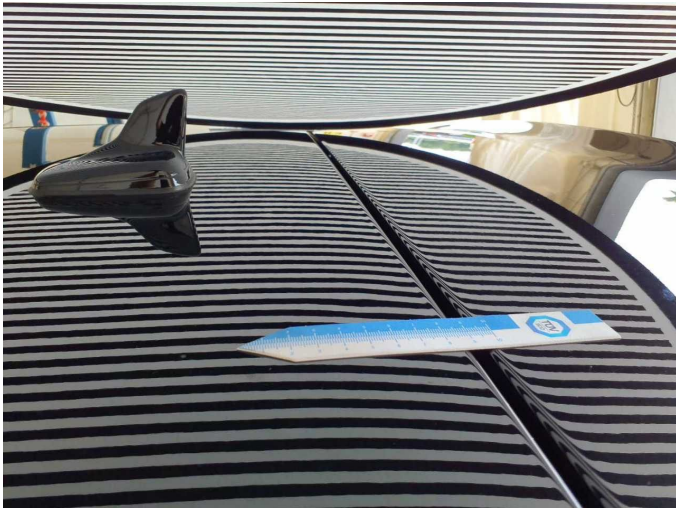
Damage 1: Roof: Roof - dent(s) - Smooth repair work
