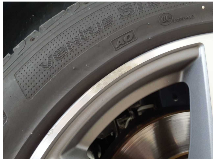
Damage 12: Wheel / tyres: Alloy rim - front right side - Corrosion - Replace
