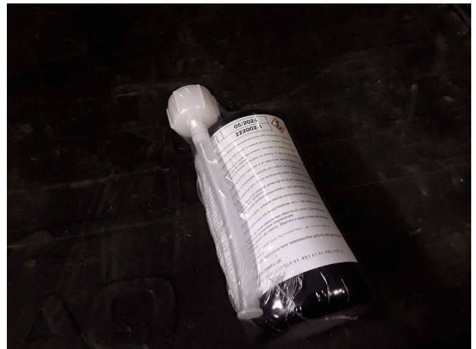
Damage 2: Equipment: Tirefit filler - Expired - Replace
