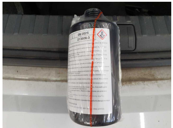
Damage 2: Equipment: Tirefit filler - Expired - Replace
