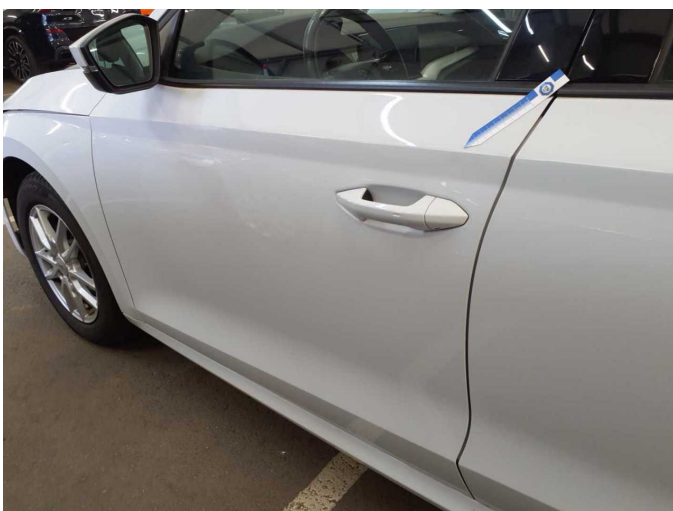
Damage 3: Door - front left side: Door - dent(s) - Smart repair
