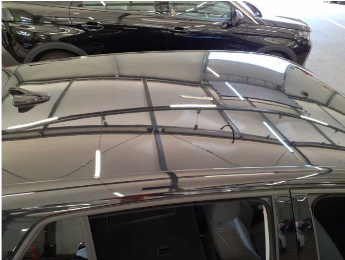
Damage 1: Roof: Roof - dent(s) - Smooth repair work
