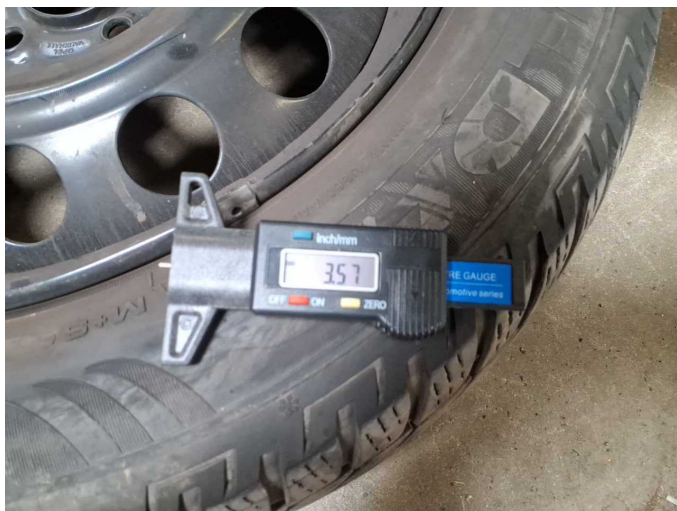
Damage 5: 2nd wheel set: 1 tyre (Rest über 4mm.) - Does not meet the leasing specifications - Replace
