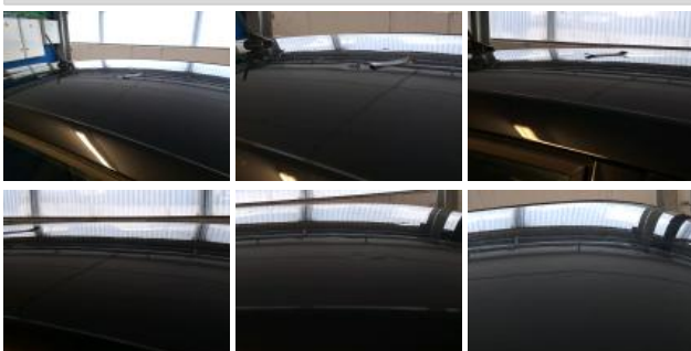
Roof, Hail damage, Repair and paint (complete)
