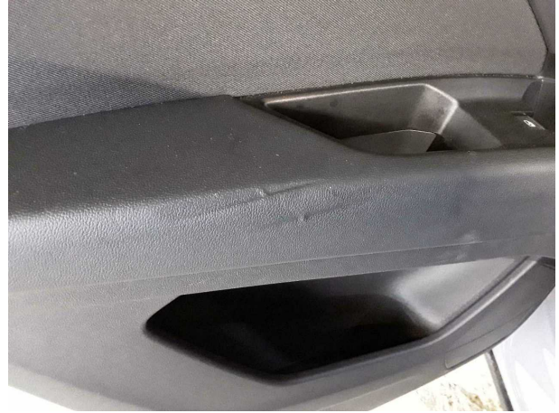
Damage #1: Trim / covers: Door trim - rear left side (Druckstellen) - No deduction
