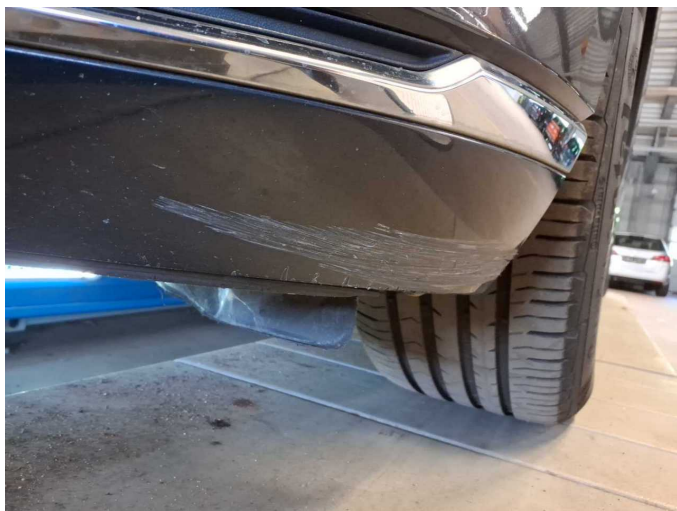
Damage 4: Front bumper: Spoiler - Scratched - Paint
