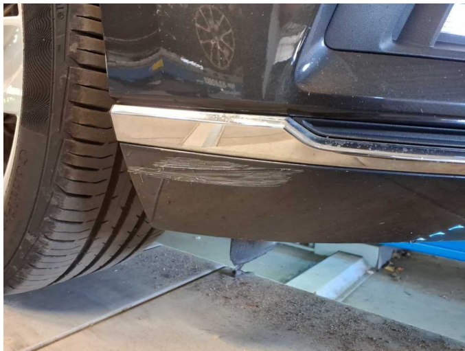
Damage 4: Front bumper: Spoiler - Scratched - Paint
