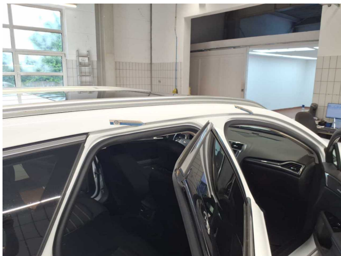
Damage 1: Roof: Roof rail - right side (Dichtstopfen) - Missing - Replace
