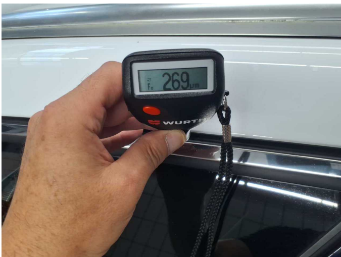
Repainting 1: Roof rail - right side
