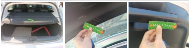
Rear bulkhead lining, Scratch(es), Repair/replace (lump sum)
