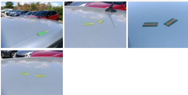
Roof, Dent(s), Repair and paint (complete)
