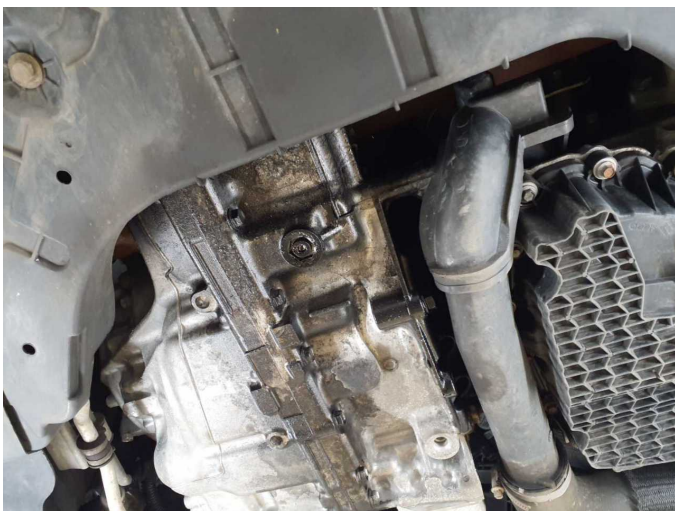
Damage 4: Engine: Engine - Leaking - Perform diagnosis
