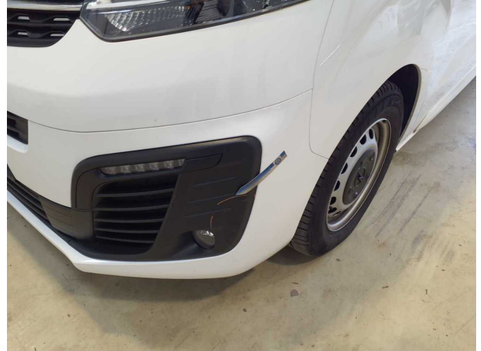
Damage 8: Front bumper: Cover bumper - front (Links) - Scratched - Replace
