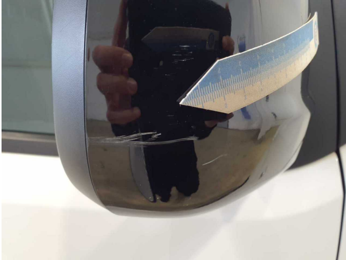
Damage 2: Wing mirror - right side: Cap - Scratched - Smart repair
