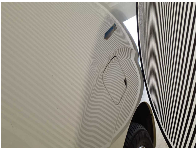
Damage 9: Side panel - rear left side: Side panel (Unterhalb) - dent(s) - Repair and paint
