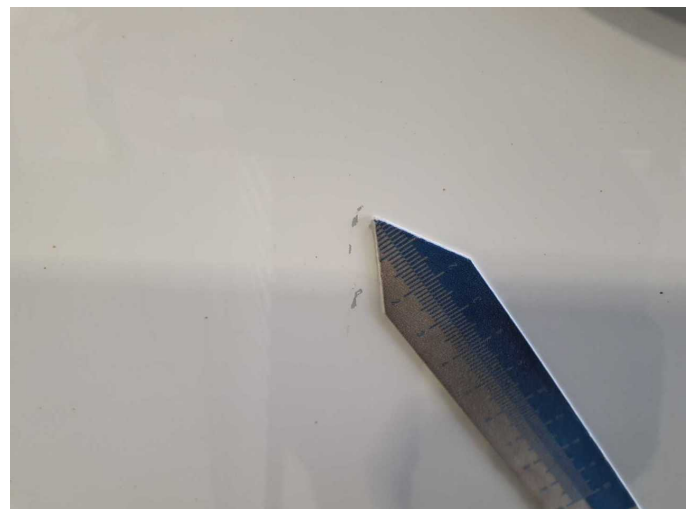
Damage 7: Door - front left side: Door - Scratch(es) - Smart repair
