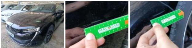
Door FR, Dent(s), Repair and paint (complete)
