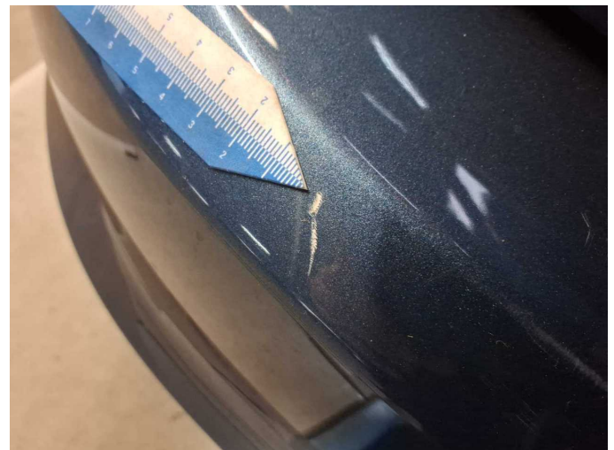
Damage 3: Rear bumper: Rear bumper (Kratzer) - Deformed - Repair and paint
