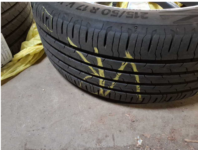
Damage 4: 2nd wheel set: 3 tyres (Lauffläche) - Damaged - Replace
