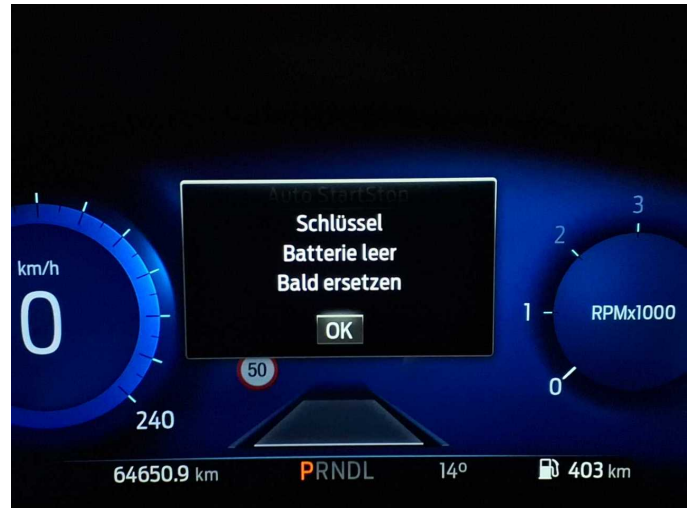
Damage 1: Equipment: Vehicle key (Batterie) - Empty - Replace
