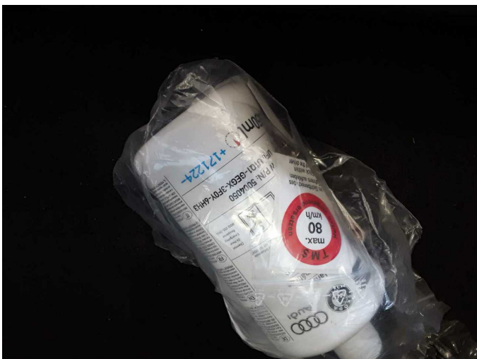
Damage 1: Equipment: Tirefit filler - Expired - Replace
