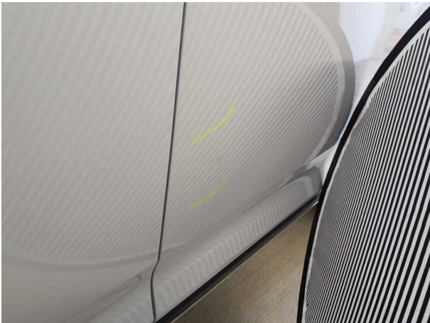
Damage #2: Door - rear left side: Door - dent(s) - Smooth repair work
