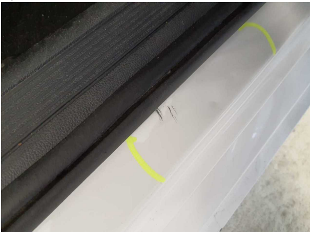
Damage #3: Sill - right side: Sill - Dent / paintcoat damage - Repair and paint
