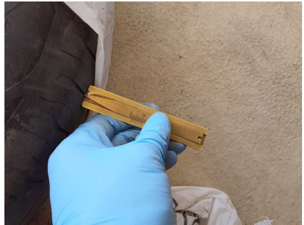
Damage #4: 2nd wheel set: Tyres - complete set - Worn - repair/paint (S1)
