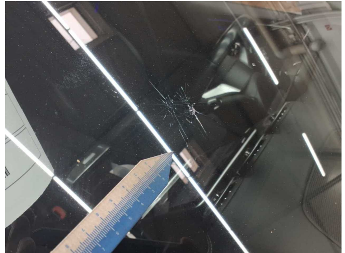
Damage 11: Vehicle glazing: Windscreen - Stone chips - Replace
