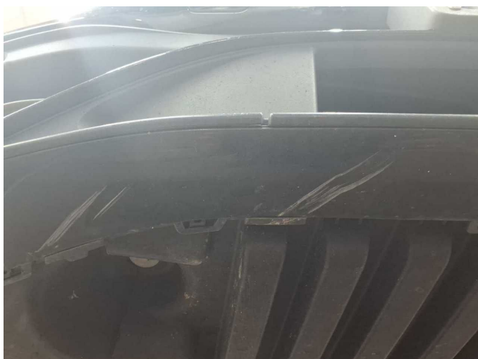
Damage 9: Front bumper: Front bumper - Scratch(es) - Paint
