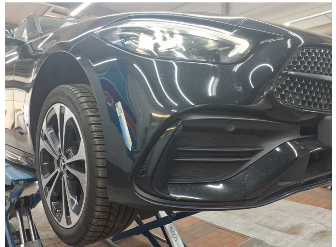
Damage 9: Front bumper: Front bumper - Scratch(es) - Paint
