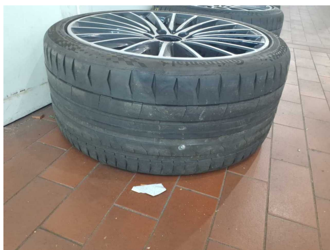
Damage 6: Wheel / tyres: Tyre - rear left side (Nagel im reifen) - Damaged - Replace
