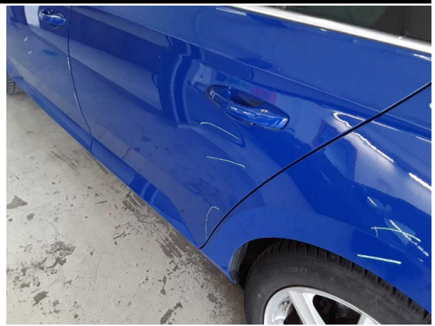
Damage #5: Door - rear left side: Door - Scratched - Repair a... paint
