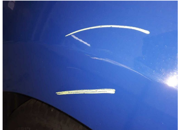
Damage #1: Side panel - rear left side: Side panel - Scratch(... - Cover / polish
