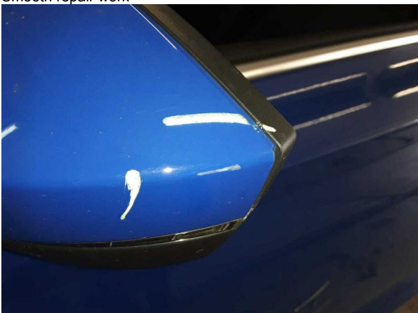
Damage #3: Wing mirror - left side: Cap - Scratched - Smart repair
