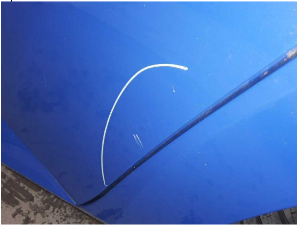
Damage #5: Door - rear left side: Door - Scratched - Repair and paint
