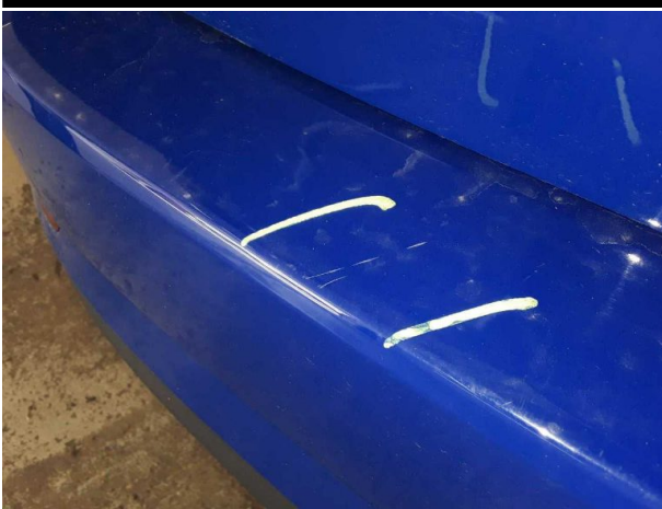
Damage #6: Rear bumper: Rear bumper - Scratched - Repair and paint
