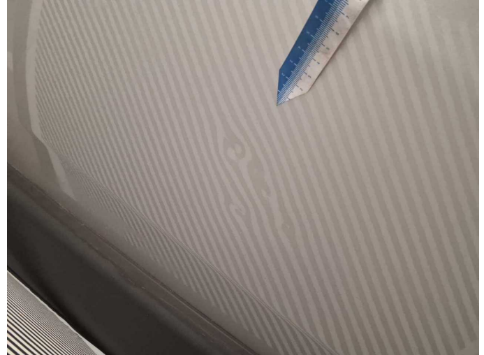
Damage 13: Boot lid / rear door: Rear door - right side - Deformed - Repair and paint
