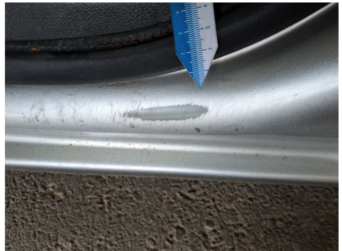
Damage 5: Sill - left side: Sill - Scratched - Smart repair
