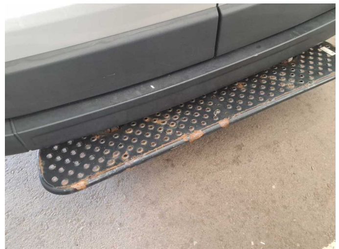
Damage 6: Rear of vehicle: Foot plate - Corrosion - Loss in value
