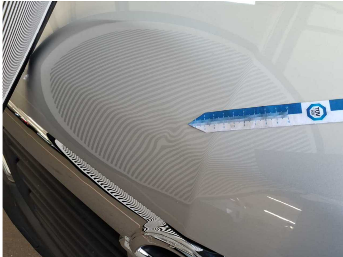
Damage 10: Bonnet: Bonnet - Deformed - Repair and paint
