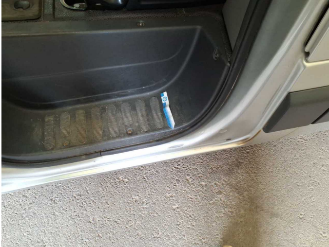
Damage 7: Door - front left side: Door seal - Damaged - Replace
