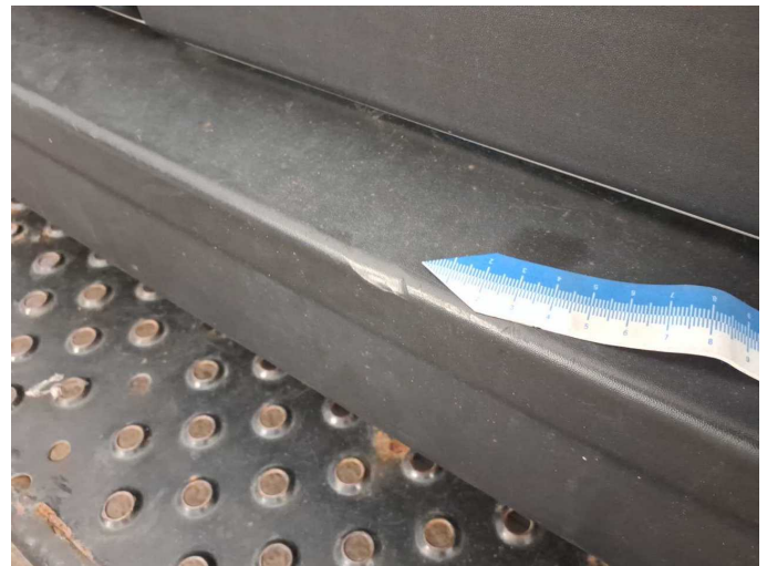
Damage 8: Rear bumper: Rear bumper - Scratched - Loss in value
