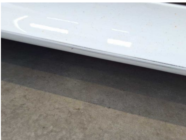
Damage #10: Sill - right side: Trim - Scratch(es) - Paint
