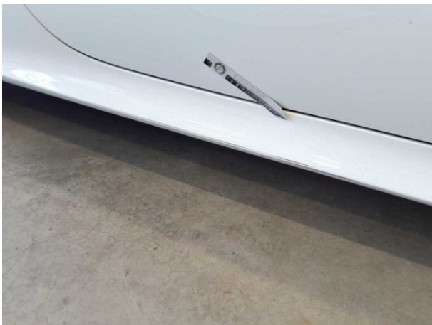
Damage #10: Sill - right side: Trim - Scratch(es) - Paint
