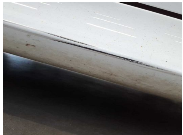
Damage #10: Sill - right side: Trim - Scratch(es) - Paint
