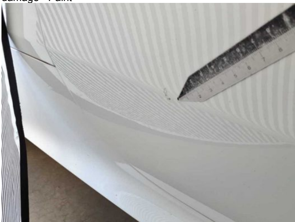
Damage #12: Door - front right side: Door - Dent / paintcoat damage - Paint
