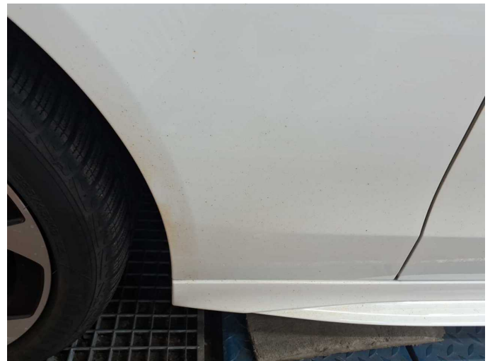
Damage 1: Body: Body (Flugrost) - Conditioning
