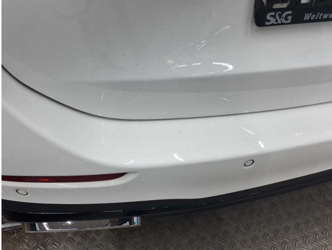
Damage 1: Body: Body (Flugrost) - Conditioning
