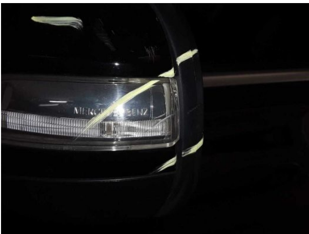
Damage #5: Indicator - front: Mirror - left side - Scratched - Replace
