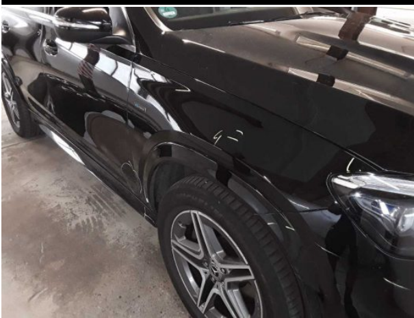
Damage #10: Mudguard - right side: Mudguard - right side - Scratched - Smart repair
