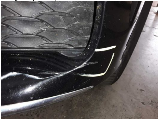
Damage #18: Front bumper: Front bumper - Deformed - Replace
