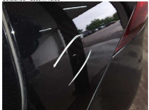
Damage #9: Side panel - rear left side: Side panel - Scratch(...) - Smart repair
