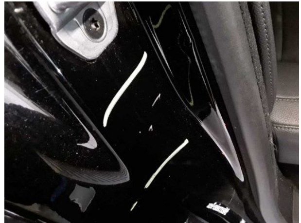
Damage #13: Sill - right side: Sill - Dent / paintcoat damage - Smart repair
