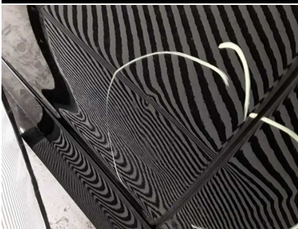
Damage #16: Door - front right side: Door - Dent / paintcoat damage - Repair and paint
