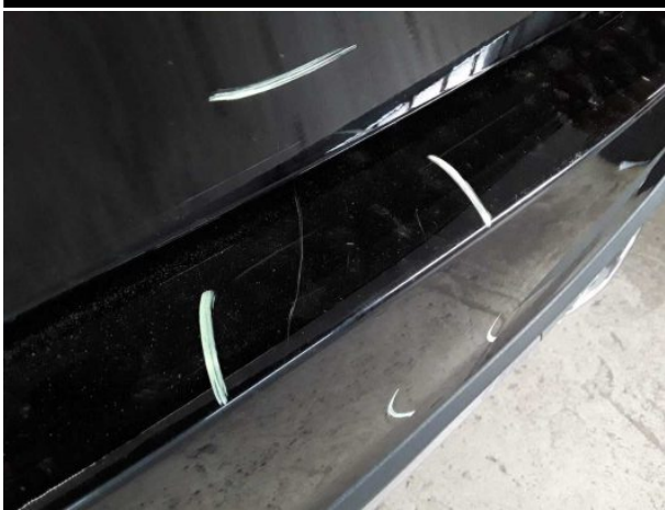
Damage #15: Rear bumper: Rear bumper - Scratched - Repair and paint
