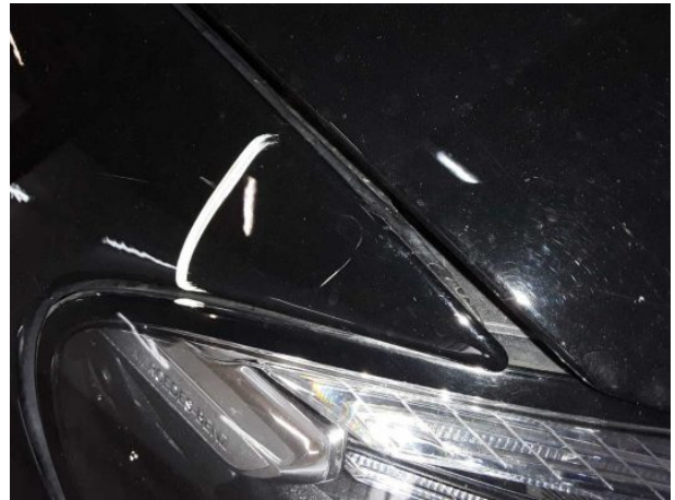
Damage #10: Mudguard - right side: Mudguard - right side - Scratched - Smart repair
