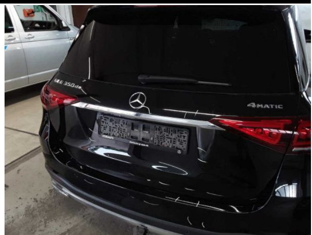
Damage #17: Boot lid / rear door: Boot lid - Dent / paintcoat damage - Repair and paint
