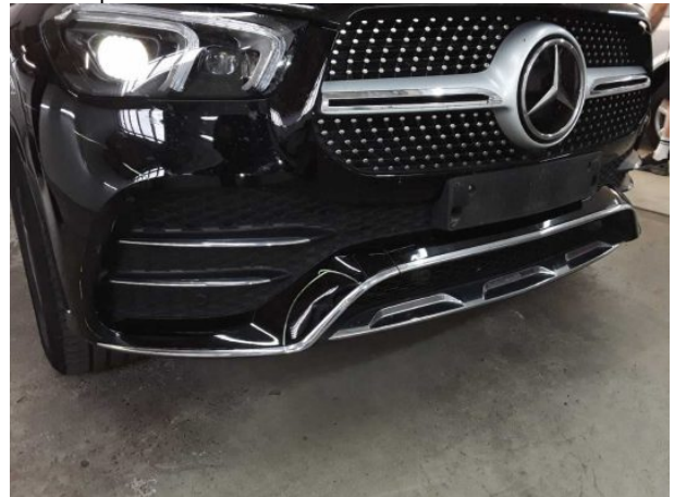
Damage #14: Front bumper: Spoiler - Scratched - Replace
