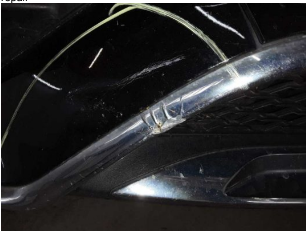
Damage #14: Front bumper: Spoiler - Scratched - Replace
