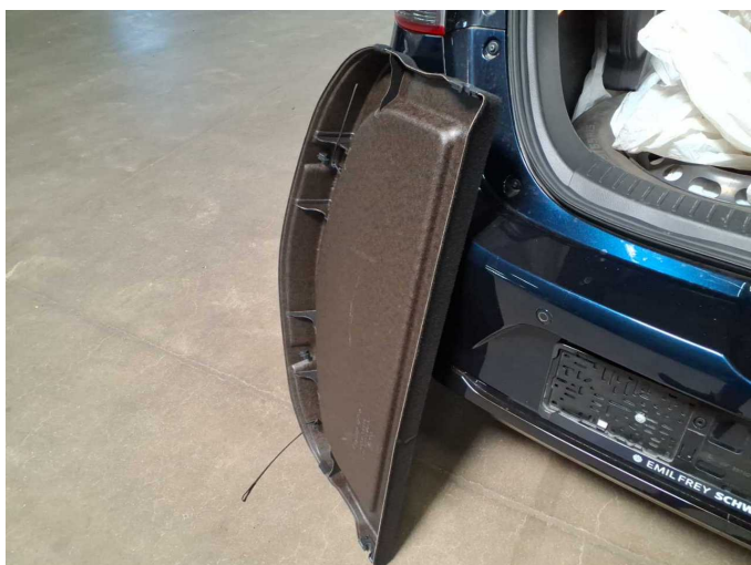
Damage 2: Interior: Rear shelf - Broken / torn - Replace
