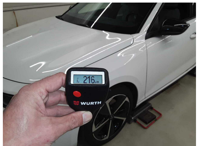
Mudguard - left side: 216 µm
