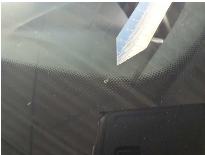
Damage 8: Vehicle glazing: Windscreen with rain sensor - Stone chips - Replace
