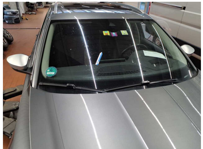
Damage 9: Vehicle glazing: Windscreen (2 x) - Stone chips - Replace
