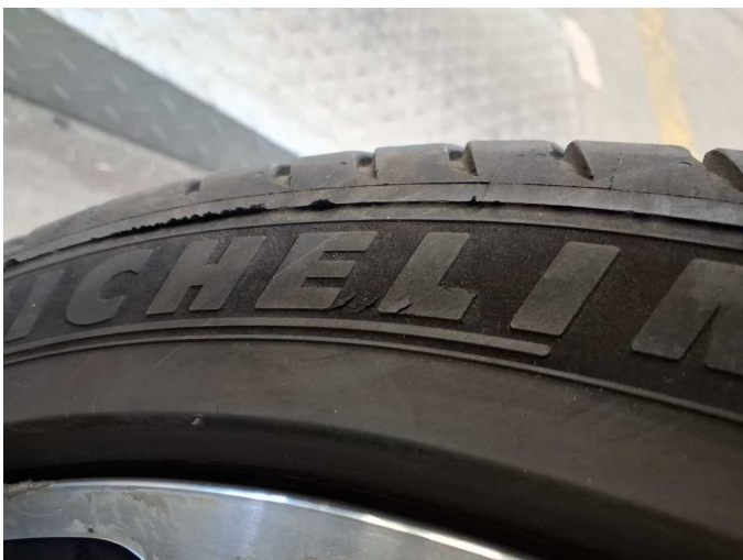
Damage 8: 2nd wheel set: 3 tyres (Flanke) - Damaged - Replace
