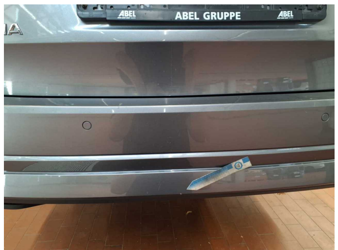
Damage 6: Rear bumper: Rear bumper - Scratched - Paint
