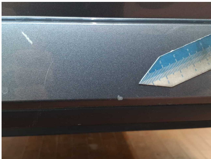
Damage 6: Rear bumper: Rear bumper - Scratched - Paint
