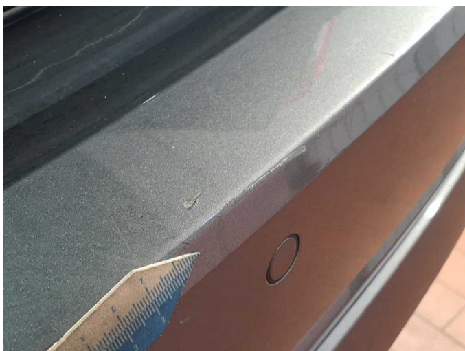
Damage 6: Rear bumper: Rear bumper - Scratched - Paint
