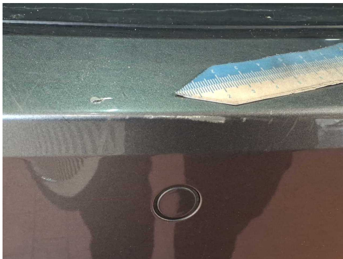
Damage 6: Rear bumper: Rear bumper - Scratched - Paint
