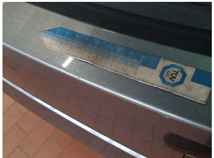
Damage 6: Rear bumper: Rear bumper - Scratched - Paint
