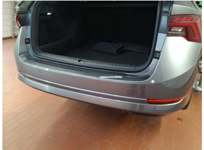
Damage 6: Rear bumper: Rear bumper - Scratched - Paint
